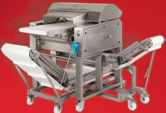
The BXM KR is suitable for continuous membrane skinning of flat cuts. The product is positioned on the infeed conveyor belt and the first side is skinned. A return conveyor sends the product back to the operator who positions the product once again on the infeed conveyor. The second side is then skinned. Membrane is collected in an Ell membrane box placed under the machine or onto a lateral discharge conveyor.
